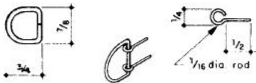
FIGURE 30. HAND SPIKE "D"-RING 1/8" Dia. Steel Rod, 2 Required
